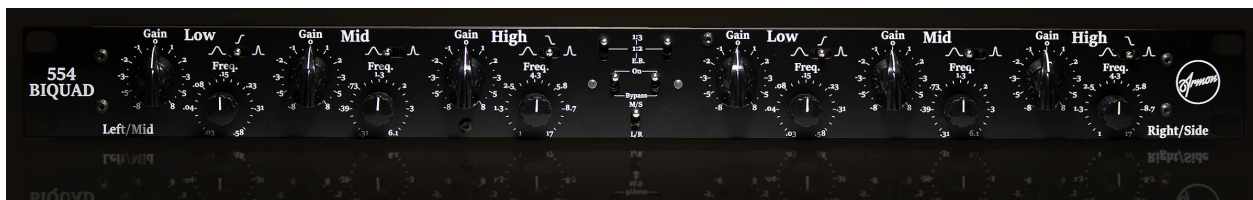
FIG. 1 The 554 Biquad front panel. Left/Mid channel on the left, Right/Side on the right, and the central switch section between them.
