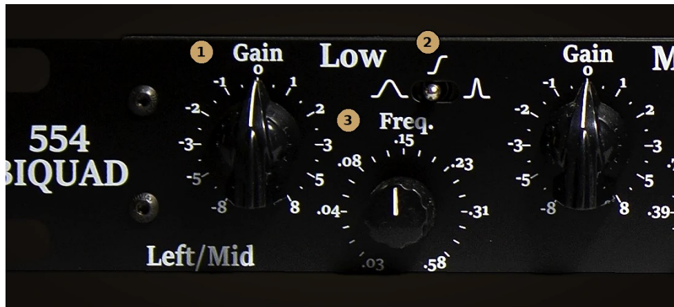
FIG. 5 Controls of one band (Low, Left/Mid): (1) Gain, (2) curve selector, (3) Freq.
