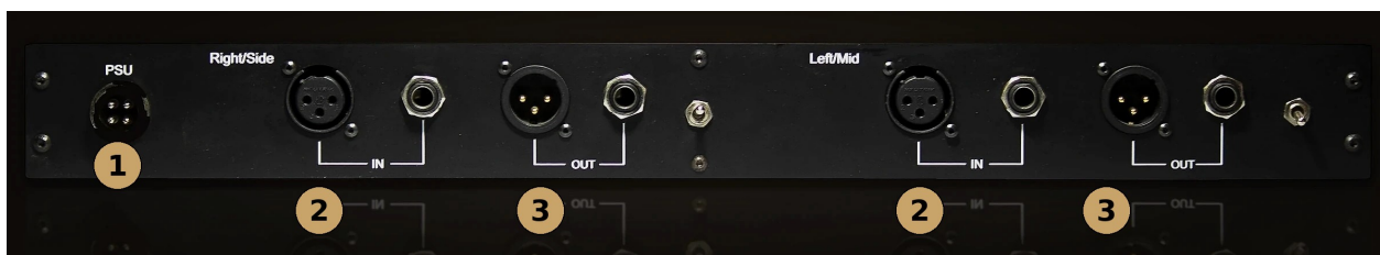
FIG. 7 Rear panel, seen from behind (Right/Side on the left, Left/Mid on the right): (1) PSU, (2) IN, (3) OUT.
